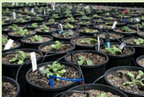
Aquaspy and ECH2O soil moisture sensors shown placed within the growing media.
