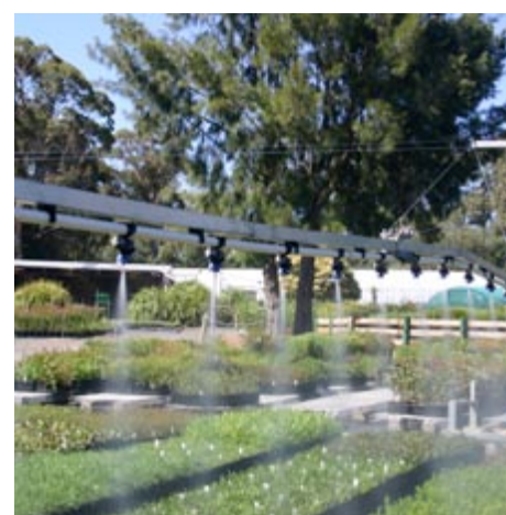
Efficient irrigation system via boom, however water use efficiency relates to how much the plant and growing media requires.
